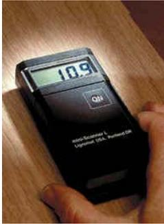
The mini-Scanners are used for measuring the moisture level in finished wood products or other building materials where it is not desirable to leave pin marks on the finished product. It indicates wet and dry moisture levels. This economically priced meter offers state-of-the-art electronics with 8 settings (32 Settings for SD model) to correct for different species. Large easy to read LCD display offers 0.1% resolution.
